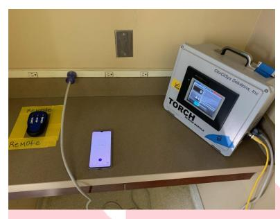
Figure 12 – Start cycle on remote. Start logging on touchscreen.
