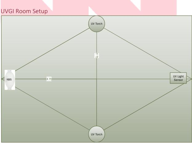
Figure 1 – Room Setup (Overhead View). The lines holding the N95 FFRs are 13 feet long and hold 30 respirators per line (3 across the room); the UVGI "torches" are located 4 feet from the center of the line and are 8 feet apart.
