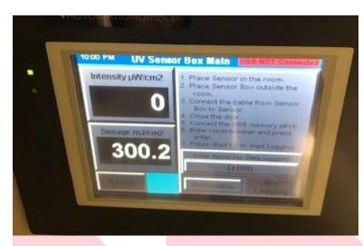
Figure 14 – Run cycle until dose is not less than 300 mJ/cm<sup>2</sup>.
